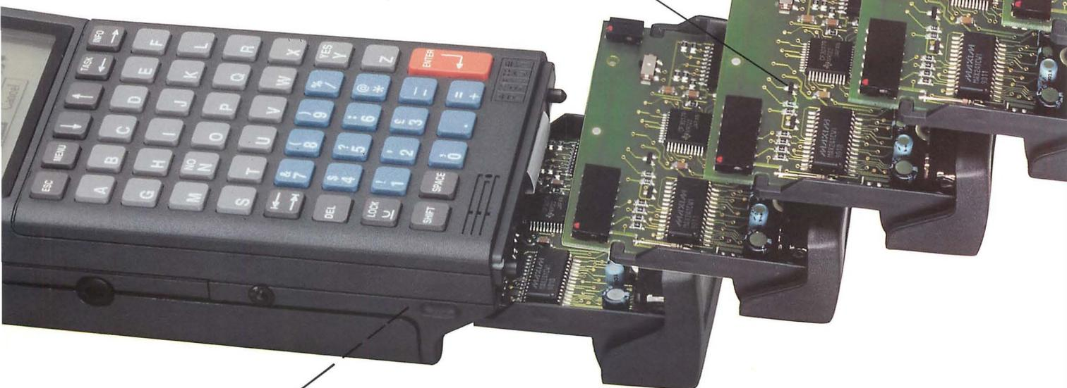
Lithium backup battery preserves the internal RAM when battery pack is removed.
