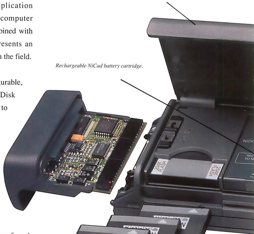
*Solid State Disks offer equivalent functionality to floppy or hard disks, but have no moving parts and are completely reliable. Using MS-DOS file format, they can plug directly into standard PCs as well as HCs, providing a simple and totally reliable data transfer mechanism. Individual capacities of up to 2 Mbytes each, rising through 1992, with two SSD drives built in as standard.*
